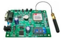
Fig 3. GPRS modem
