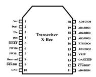
Fig 4. ZIGBEE pin diagram
